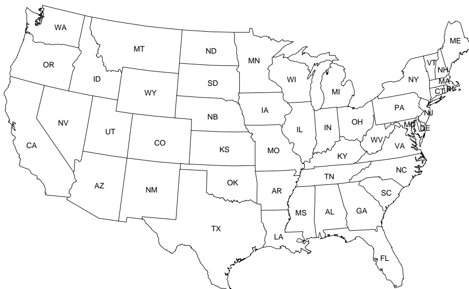
Figure 8. An equal area Albers projection of the USA with true scale at latitudes 30^\circ and 40^\circ .
