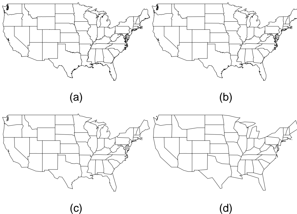
Figure 9. State map drawn at four resolutions: 0, 1, 5, and 20 respectively. The first map shows all the data in the state database, the second is adjusted to expunge consecutive points that are within a printer pixel of each other, while the remaining two pictures do the same thing for points within 5 and 20 pixels of each other. The number of coordinate pairs defining these four maps is 11519, 3208, 1066 and 681, respectively.
